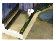
Fig. 5-12: Lubricated support profiles
